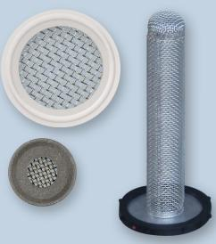
Rubber Fab's fluid filtration screen gaskets provide the most comprehensive range of stainless steel mesh and filter cloth. These gaskets provide particulate elimination to protect fill and finish sterile products, spray balls and spray nozzles. You can choose a screen gasket in a USP Class VI elastomer or Fluoroelastomer and are available in a variety of mesh sizes including 10 micron through 4 mesh. Custom screens are also available.
