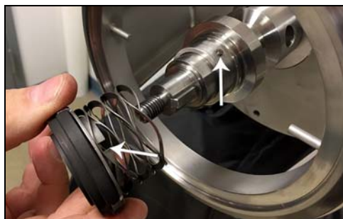
Figure 66 - Remove seal, cup, and spring
