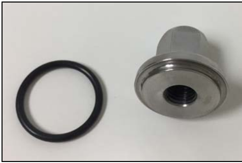
Figure 108 - Install O-ring on impeller nut
