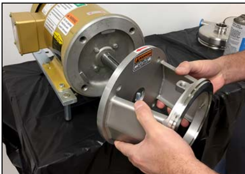
Figure 75 - Remove motor adapter
