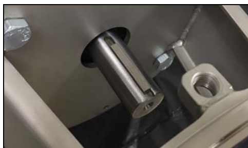
Figure 29 - Install key in motor shaft
