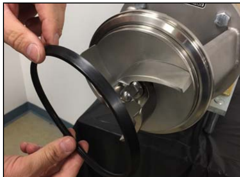
Figure 59 - Remove casing gasket
