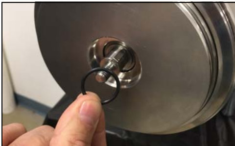
Figure 64 - Remove stub shaft O-ring
