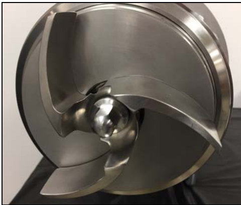
Figure 110 - Hand-tighten impeller nut
