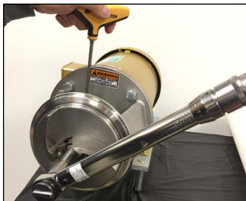
Figure 60 - Loosen impeller nut
