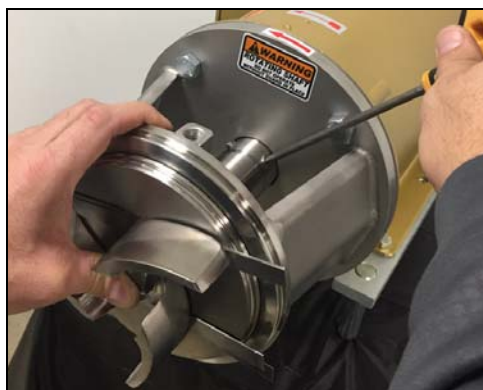
Figure 37 - Place feeler gauge, tighten setscrews
