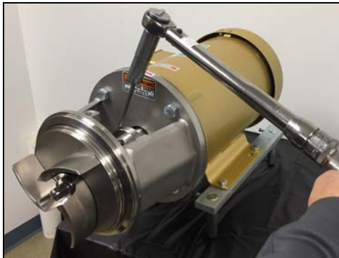
Figure 92 - Torque drive collar screws
