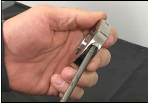
Figure 79 - Remove drive collar screws
