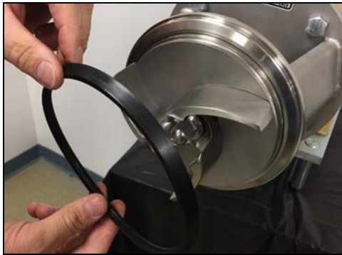
Figure 112 - Place casing gasket onto backplate
