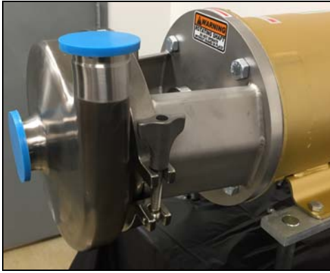
Figure 116 - Hand-tighten casing clamp
