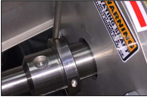
Figure 72 - Loosen shaft collar screws
