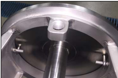
Figure 32 - Backplate pins engaged with adapter pins
