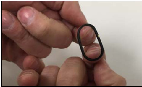
Figure 104 - Lightly stretch O-ring
