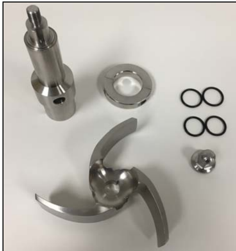
Figure 76 - Sealed Impeller Components (Note: only one set of O-rings is required)
