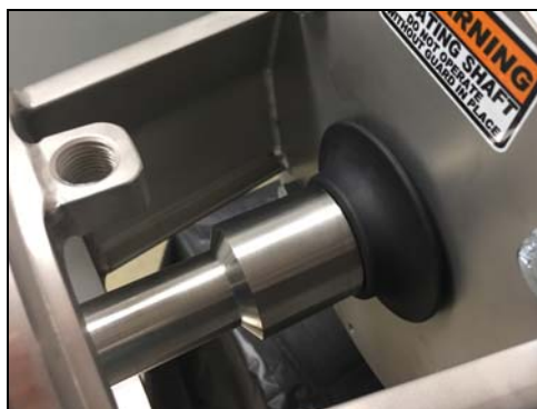
Figure 38 - Slide deflector onto shaft
