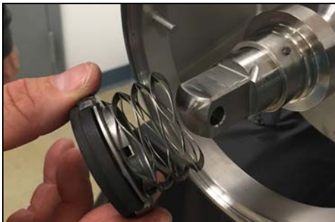
Figure 19 - Remove seal, O-ring, seal cup and spring
