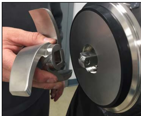
Figure 35 - Slide impeller on shaft
