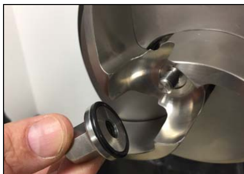
Figure 61 - Remove impeller nut
