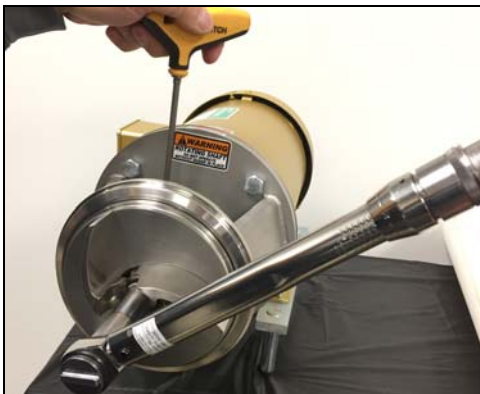
Figure 111 - Torque impeller nut
