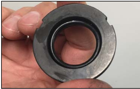
Figure 43 - Seal O-ring installed
