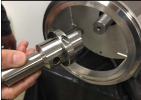
Figure 73 - Slide stub shaft off motor shaft
