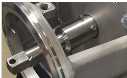
Figure 30 - Stub shaft on motor shaft
