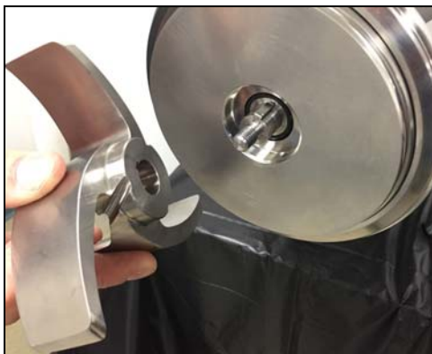
Figure 107 - Install impeller on stub shaft
