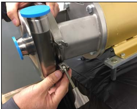
Figure 115 - Install casing clamp
