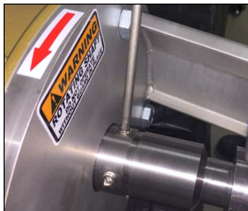
Figure 23 - Pin Impeller: Loosen setscrews
