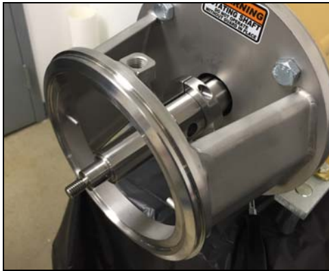
Figure 83 - Stub shaft on motor shaft
