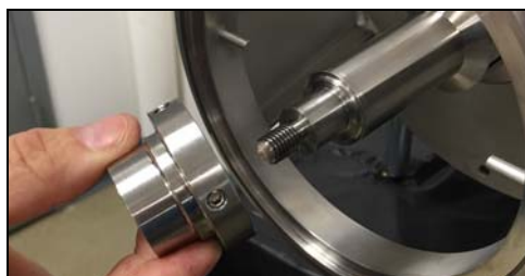
Figure 71 - Remove drive collar
