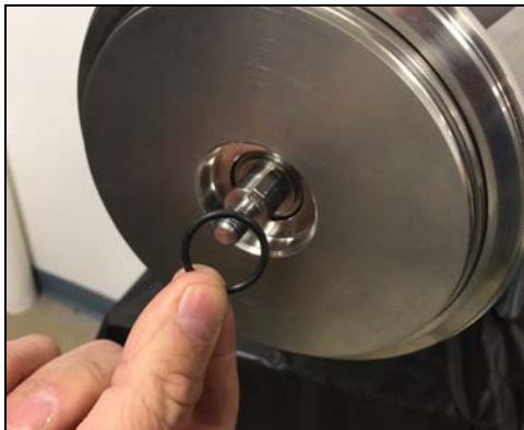
Figure 105 - Install stub shaft O-ring
