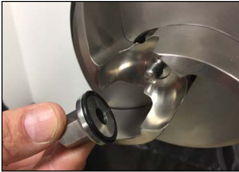
Figure 109 - Install impeller nut
