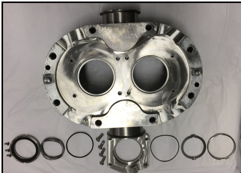
Figure 83 - Double Mechanical Seal (040-U3 shown)
