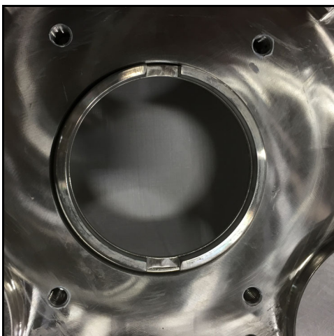
Figure 85 - Shaft ring installed
