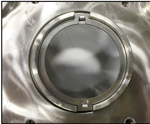
Figure 87 - Drive ring installed
