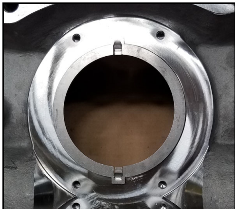
Figure 64 - Drive ring installed
