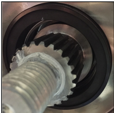
Figure 137 - Stationary seal installed
