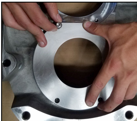
Figure 67 - Install seal housing bolts
