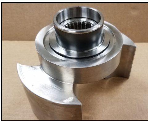
Figure 176 - Seal sleeve installed
