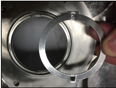
Figure 81 - Remove drive ring
