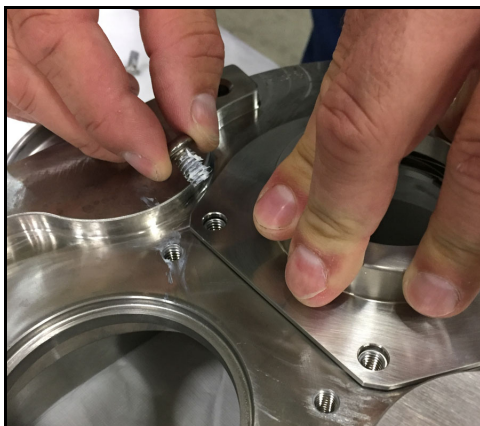
Figure 61 - Install seal housing bolts
