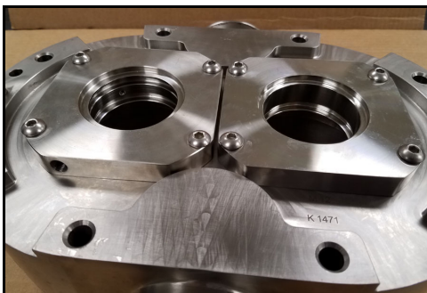
Figure 162 - Seal housings installed
