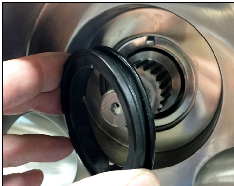
Figure 43 - Remove stationary seal
