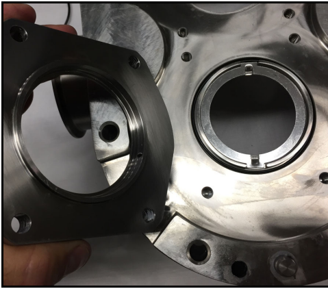
Figure 90 - Install seal housing
