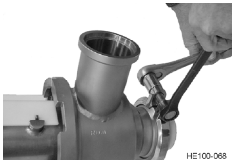
Figure 38 - Installation of Hinged Clamp
