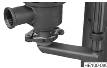
Figure 45 - Head Installed on Pin
