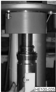
Figure 71 - Exposing Top Mechanical Seal
