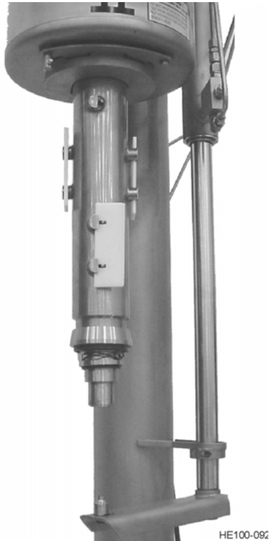
Figure 75 - Shaft With Head Removed
