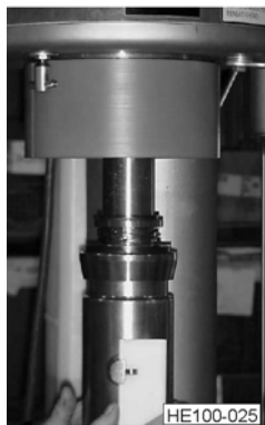
Figure 47 - Blade Alignment Tool Installed
